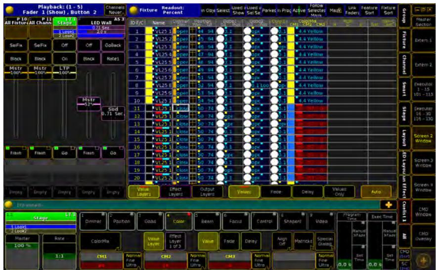
The grandMA2 onPC software incorporates all functions of a grandMA2 console and offers you its full potential on your notebook or PC. You can use grandMA2 onPC for running, programming or offline pre-programming, as well as a smart backup solution within the grandMA2 system.
