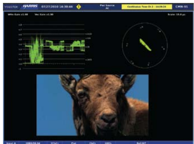
Compact Monitor Series screen capture in Overlay mode with waveform, vector and PiP display. Each component of the display is individually resizable.
