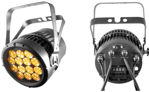
COLORado™ 2-Quad Zoom IP is one of the most powerful Par-style washes in the COLORado™ IP family, featuring 14 quad-color (RGBW) LEDs for maximum color mixing. The incorporation of wide-range zoom and 16-bit dimming curves lends considerable flexibility to designers who can use the same fixtures to highlight specific areas and flood a stage. IP-66 rated connections and hardware ensure a long life, even when exposed to the elements.
