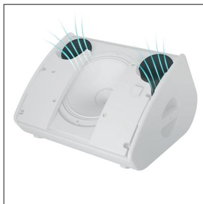
► The L-Vents laminar vented ports reduce turbulence and port noise at high levels, increasing LF efficiency.
