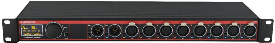
XPD-28 splitters boost, refresh and distribute the DMX signals of two inputs onto eight outputs. This allows for safely going beyond the 32 devices limit of the DMX standard, as well as for building star topologies. Moreover, the XPD-28 can be used as a repeater in order to transport a DMX signal across larger distances just as well.
