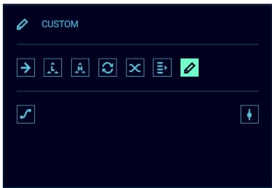
This mode is ideal for complex setup, or when per channel control is needed. Custom offers you to choose what policy to apply for each channel of each universe, and also to create a complete custom soft patch. By more, the merging policy can be remotely triggered by
