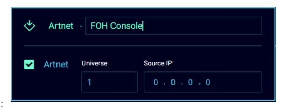
number you wish to use, and you can specify the IP address of the source as well. If you don't know the IP address of the source, simply leave the field with 0.0.0.0 IP address. The LumiNode's processing engine will bound this input to the first source using this universe number.
