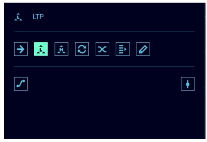
Latest Takes Precedence merging policy is commonly used to merge fixture channels. Up to 4 sources (Art-Net, sACN, DMX or RTTrPL) can be merged.
