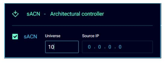
don't know the IP address of the source, simply leave the field with 0.0.0.0 IP address. The LumiNode's processing engine will bound this input to the first source using this universe number.
