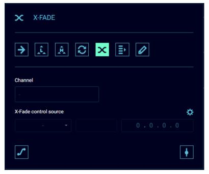
This mode offers to you to cross fade between two sources. Ideal in a situation where you need to cross fade between a lighting desk and a media server, the control channel allows you to keep full control on the speed and smoothness of the transition.
