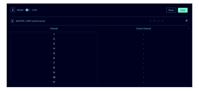
First select the mode you wish to use, by clicking on the Master Limit switch, on the upper left hand-side of the panel.
