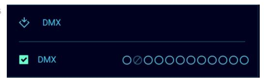
Simply tick on the port you wish to use as an input port, to enable the DMX input. A greyed-out port with a bar in the middle means this port is already used.
