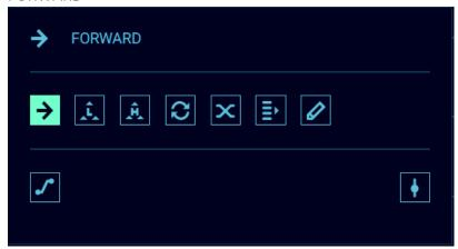
In forward mode one input source gets sent to up to 3 outputs. You can simply output to a physical port on the converter or forward to another Art-Net or sACN universe.
