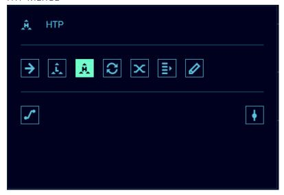
Highest Takes Precedence merging policy is commonly used to merge dimmer channels. Up to 4 sources (Art–Net, sACN, DMX or RTTrPL) can be merged.
