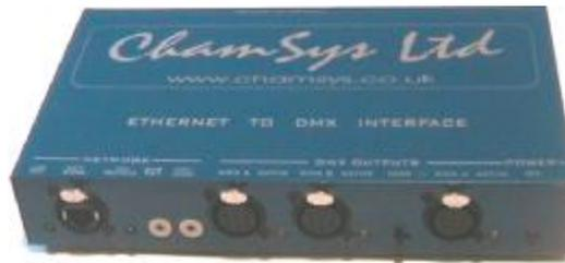
If you are using Ethernet to DMX512 conversion boxes then you will need to configure the boxes to respond to the correct ArtNet sub-net and ArtNet universe. With ChamSys 3 Universe Ethernet to DMX boxes you need to set up the two rotary switches to the correct values – the left one for ArtNet sub-net and the right one for ArtNet universe. The interface will then decode the three ArtNet universes starting from that ArtNet subnet and universe.
