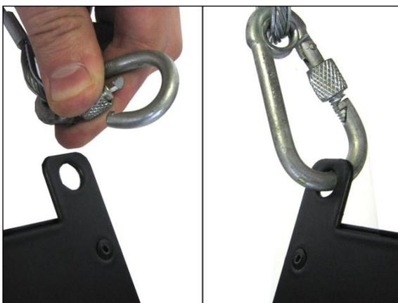
Always use an approved safety cable when attaching a Power Drop so as to secure the Power Drop to the truss or scaff pipe.
