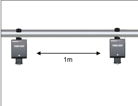
Take the width of your cloth or object that has to be dropped and determine where the first and last Power Drop have to be suspended.
