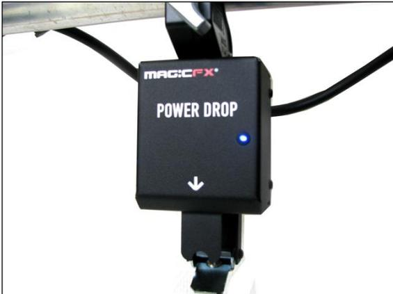
Connect the Power Drops to a 230v electricity source to check if all Power Drops have been connected properly. When everything is connected properly the blue LED indicators will light up on the Power Drops.
