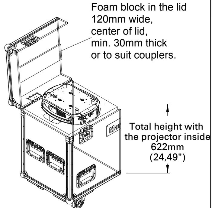
The SiP must be inserted in a flight case.
