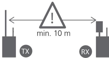
**i** Because of the signal strength, the minimum distance of 10 m between TX and RX should be maintained for the connection process. For shorter distances the directional antenna of the receiver should be shifted slightly.
