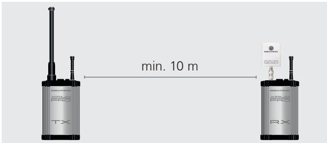
For a setup with a single transmitter and a number of receivers the minimum distance between the TX and any RX should be 10 meter.
