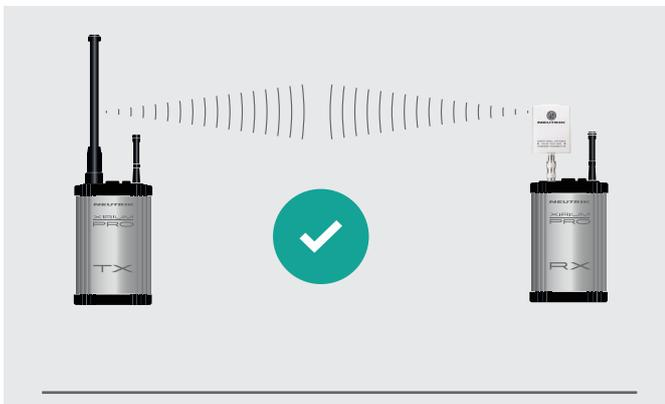
► Always mount the devices so the device antennas are at the same height.
