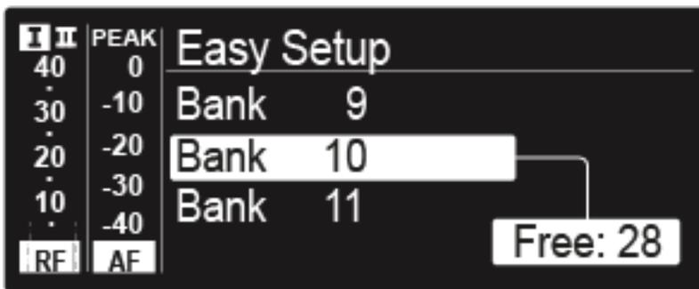
After you make your selection, the display panels of the other receivers will display the message [Assign New Frequency?](#). Receivers with non-compatible frequency ranges will display the message [Unassignable Frequency!](#).
