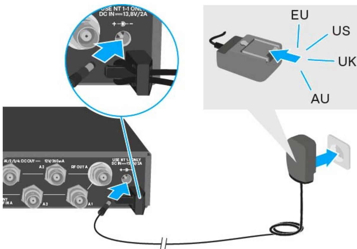
To completely disconnect the ASA 214 antenna splitter from the power supply system:
