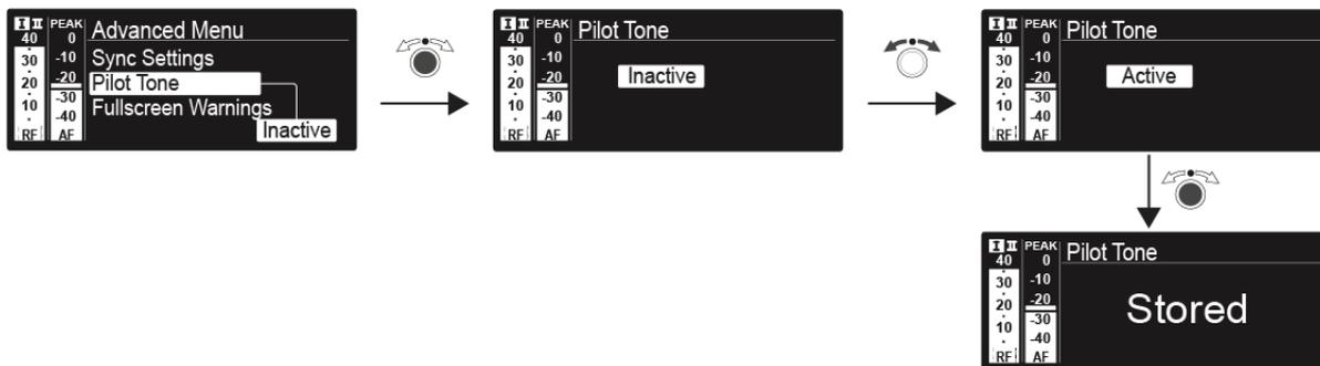
The pilot tone has an inaudible frequency that is sent from the transmitter and evaluated by the receiver. It supports the receiver's squelch function.
