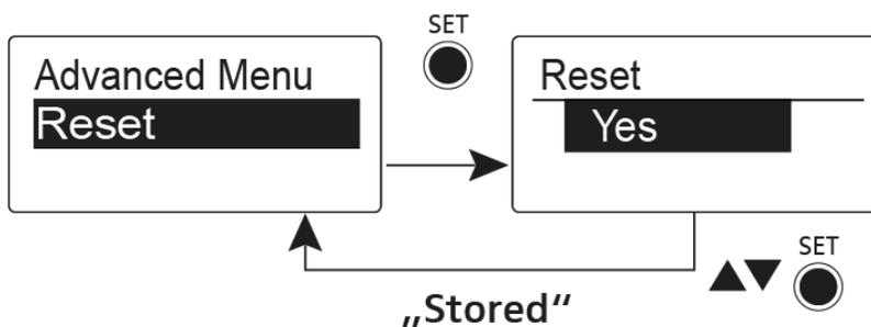
When you reset the bodypack transmitter, only the selected settings of the pilot tone and the **U** frequency bank are retained.
