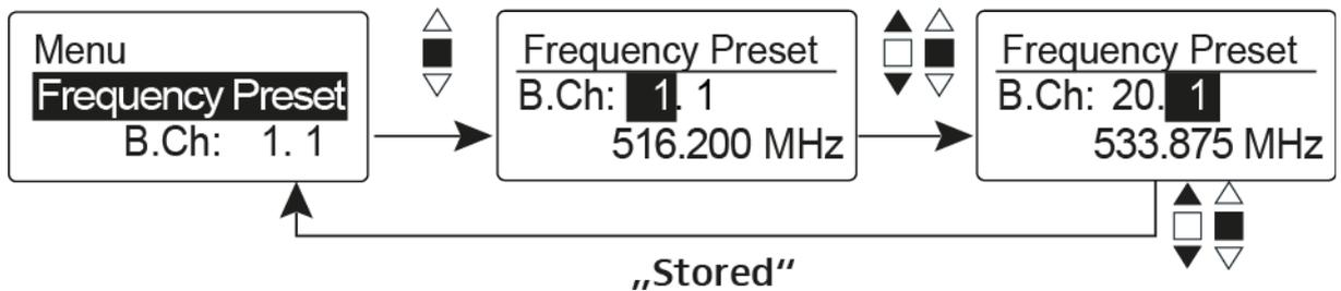
**i** While you work in the **Frequency Preset** menu, the RF signal is deactivated.
