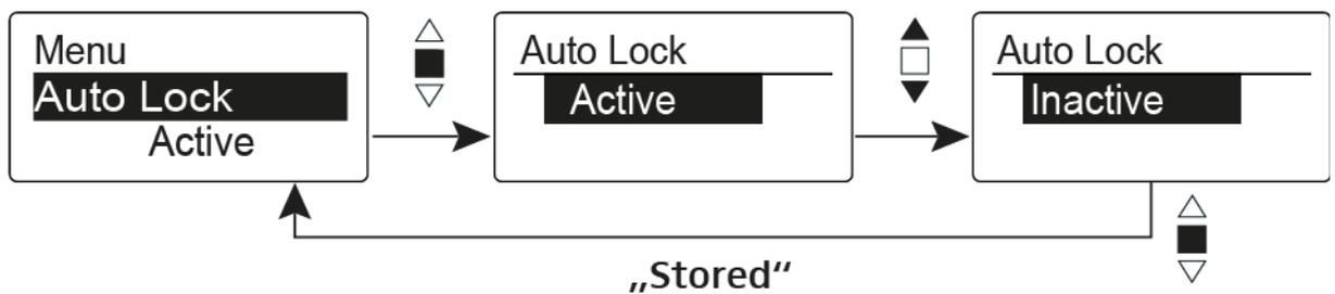
This lock prevents the wireless microphone from being unintentionally switched off and also prevents any unintentional changes to the transmitter's configuration. In the current standard display, the lock icon shows whether the lock-off function is currently switched on.
