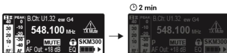
The display is dimmed automatically after 2 minutes of inactivity.
