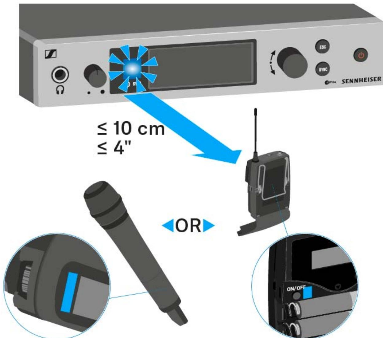
The parameters are transferred to the transmitter. The blue LED blinks during transmission.
