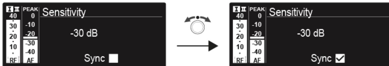
When the check box is activated, the value will be transmitted during synchronization. If it is deactivated, the value will not be transmitted.
