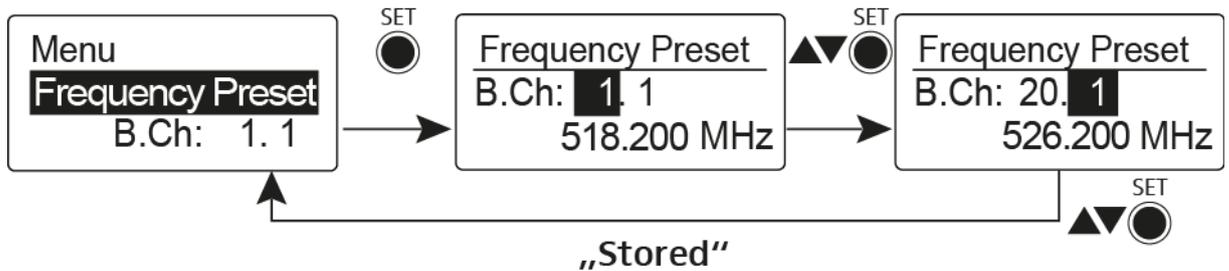
**i** While you work in the **Frequency Preset** menu, the RF signal is deactivated.
