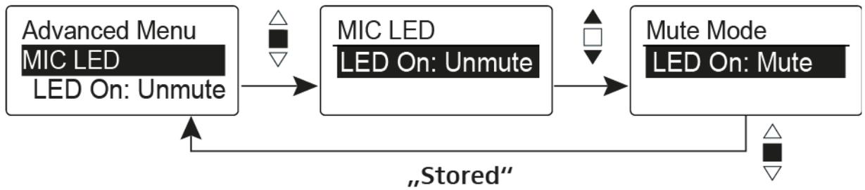
In the **MIC LED** menu item you can configure and deactivate the background lighting of the **MIC** button regardless of the settings of the “Advanced > Mute Mode menu item” and the status of the RF signal.
