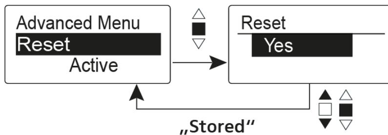
When you reset the wireless microphone, only the selected settings of the pilot tone and the **U1** to **U6** frequency banks are retained.
