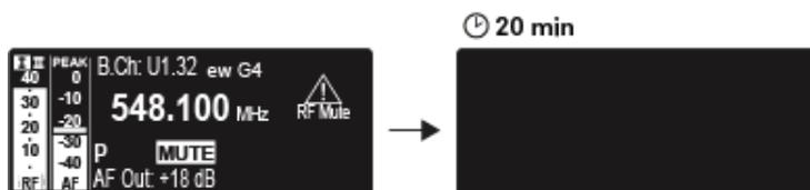
If there is no radio link to a transmitter, the display switches off after 20 minutes. The display can be reactivated by pressing any button.
