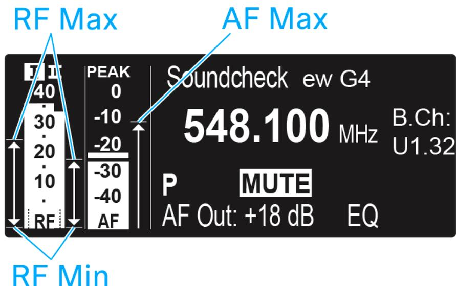
By doing a soundcheck, you can ensure adequate transmission quality in the entire area in which you want to use the transmitter. You can do the soundcheck without the help of another person.
