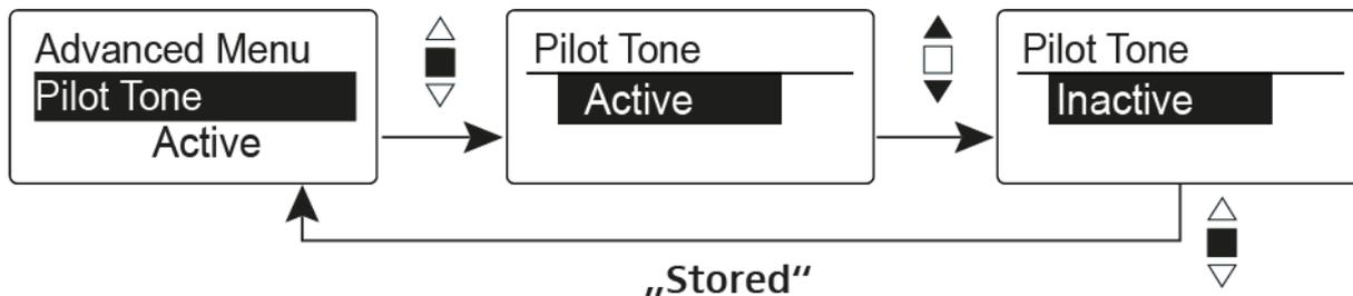
The pilot tone has an inaudible frequency that is sent from the transmitter and evaluated by the receiver. It supports the receiver's squelch function.
