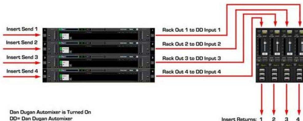
All available Outs are routed through the Dugan Automixer consecutively, thus Rack Outs routing values are identical to Automixer's channel number: Rack 1 Mono Out 1 connects to Automixer channel 1, Rack 2 Stereo Outs 3-4 connect to Automixer channels 3 and 4.
