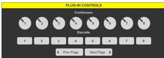
You can assign control of a Rack's Input and Output Gain, as well as Rack On/Off, Rack In/Out and Mute.
