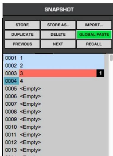
Note that selected Snapshots are highlighted, and the currently recalled Snapshot's name appears in boldface and its number is highlighted in green. At the bottom of the pane is an area where you can write notes about the selected Snapshot. To recall a Snapshot, you can either double-click on its name, or select the Snapshot and then click **Recall**.
